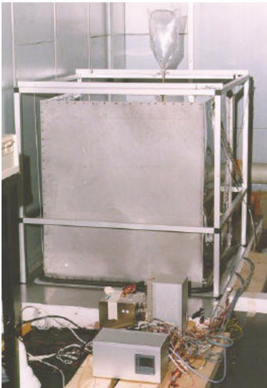
*Figure 1. The climate chamber. It stands about 1 metre high. The control electronics is in the foreground.*
